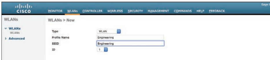
Figure 4-30 Creating a New WLAN
