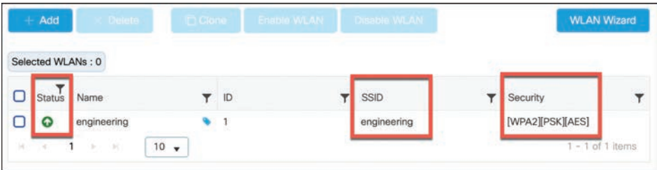
Figure 4-19 Verifying the WLAN Configuration
