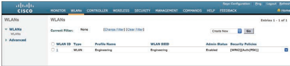
Figure 4-36 Displaying WLANs Configured on a Controller
