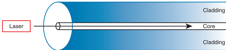
Figure 2-16 Transmission on Single-Mode Fiber with Laser Transmitter
